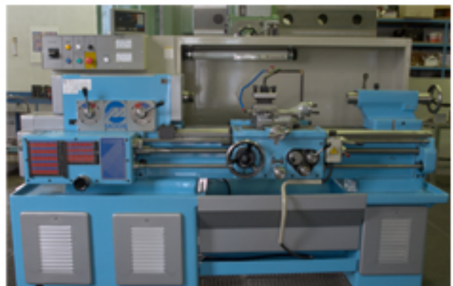
SV 18 after general repair with digital read out Newall
