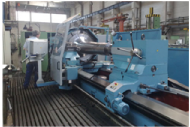
The same lathe after rebuilding SU 125 CNC with HEIDENHAIN Manualplus 4110
