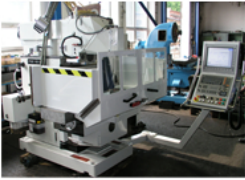
Milling machine FGS 40 CNC with HEIDENHAIN iTNC 530
