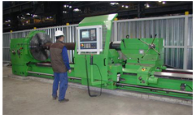
The same lathe after rebuilding SU 125 CNC with SIEMENS SINURIK 840D in plant VVT Vítkovice
